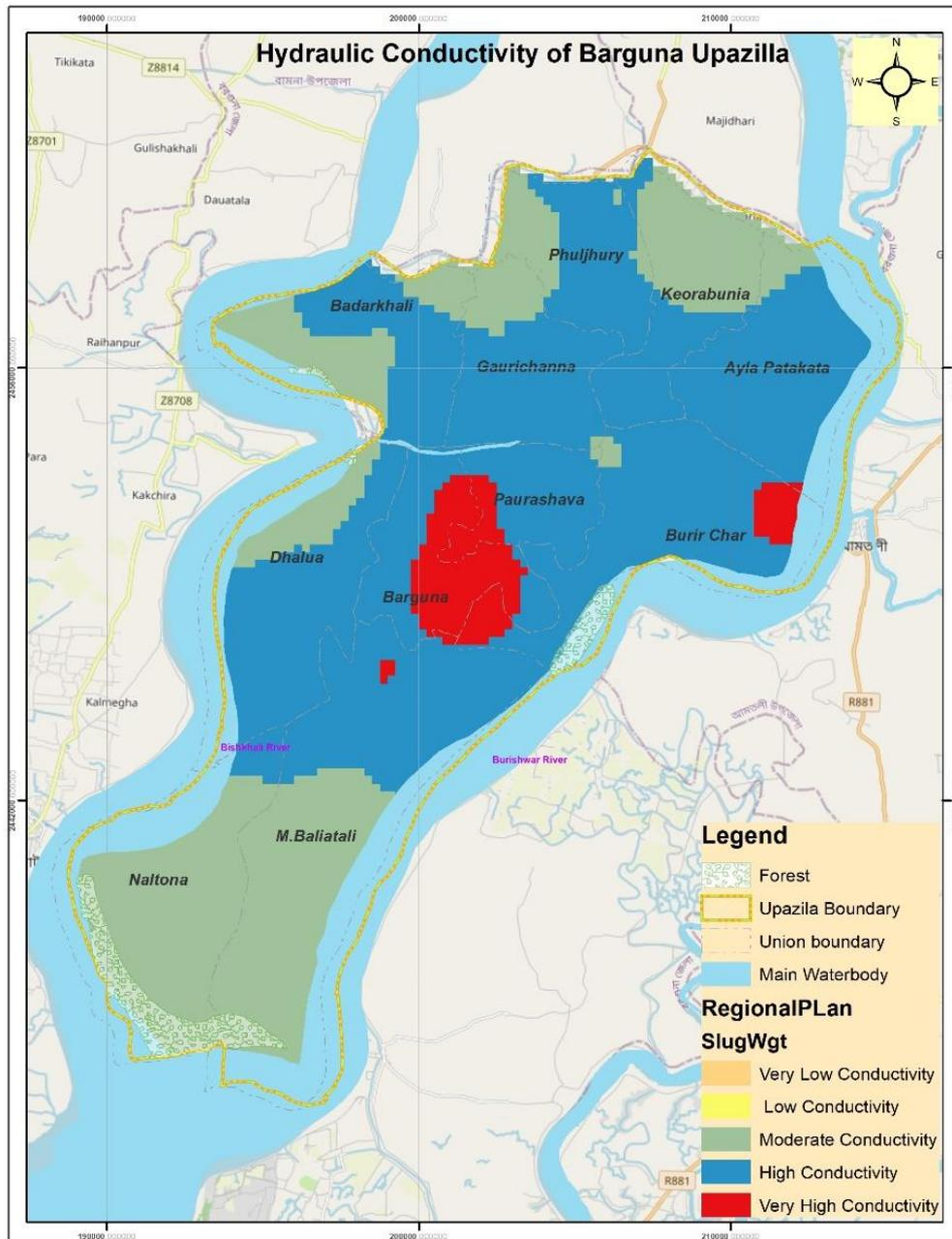
Figure 31: Hydraulic conductivity of Barguna Upazila from Slug test
