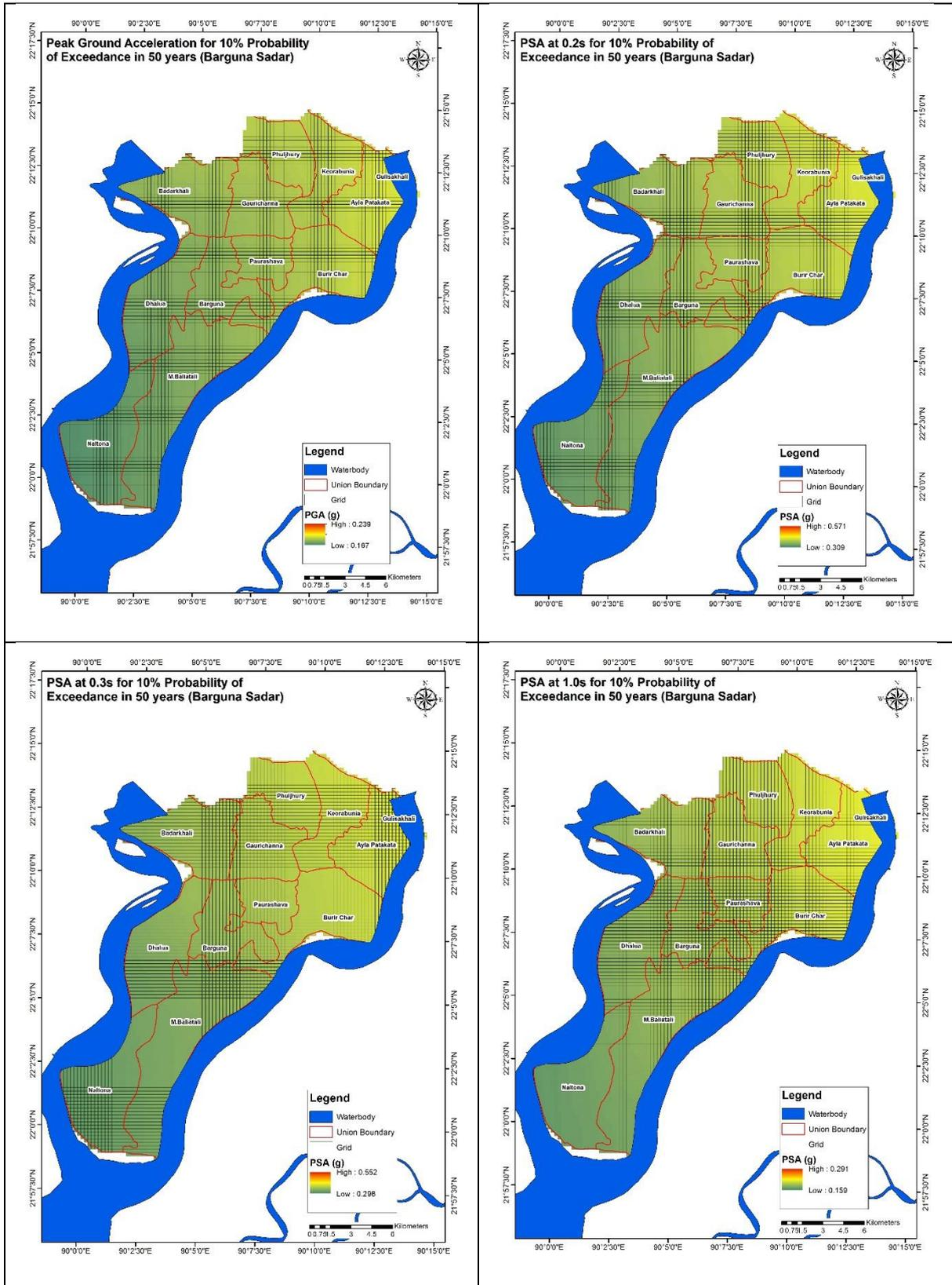
Figure 15: Probabilistic Seismic Hazard Assessment (PSHA): PGA and PSA
