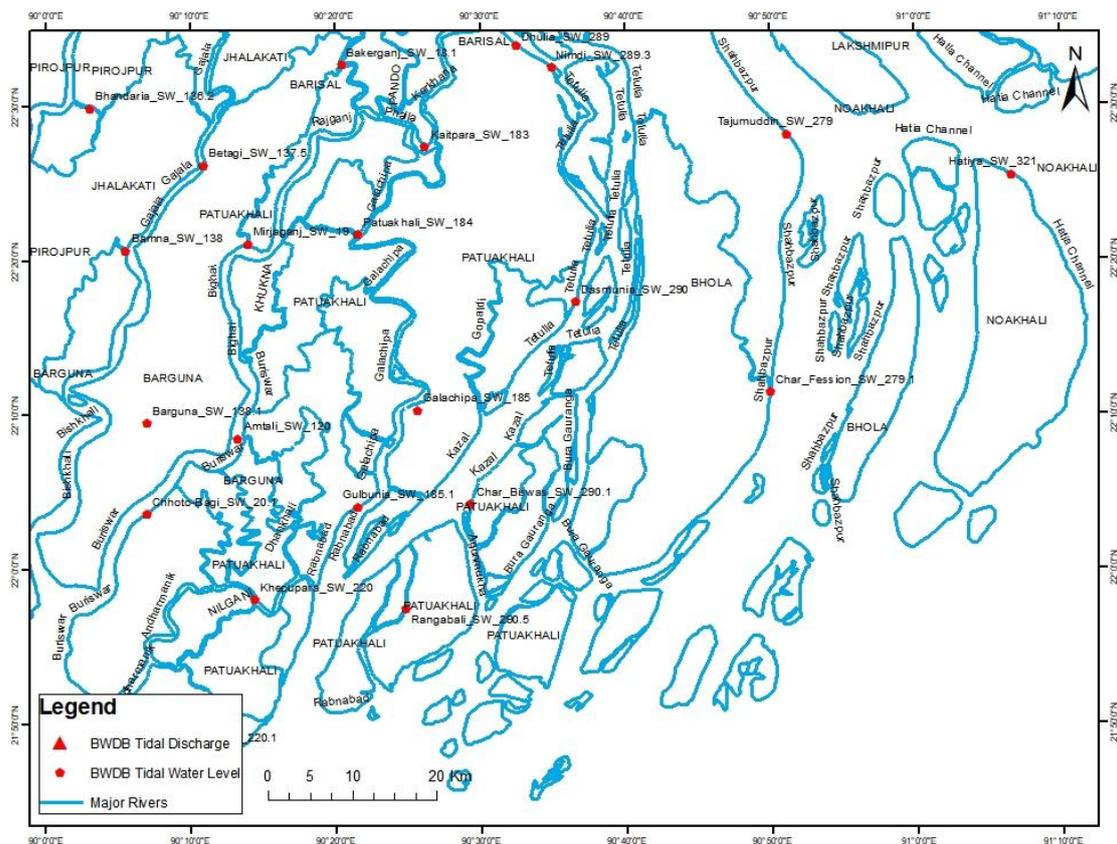
Figure 13 Location of Surface Water Gauge Station for collecting water level and discharge.
